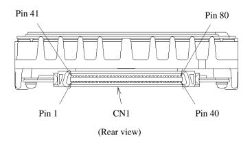
Figure A.1 Locations of connector (MC model)
